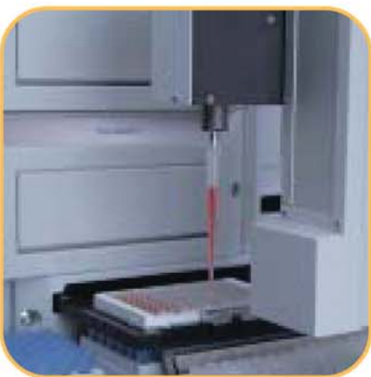
The DSX robotic arm moves microplates and pipettes all sample and reagents.
